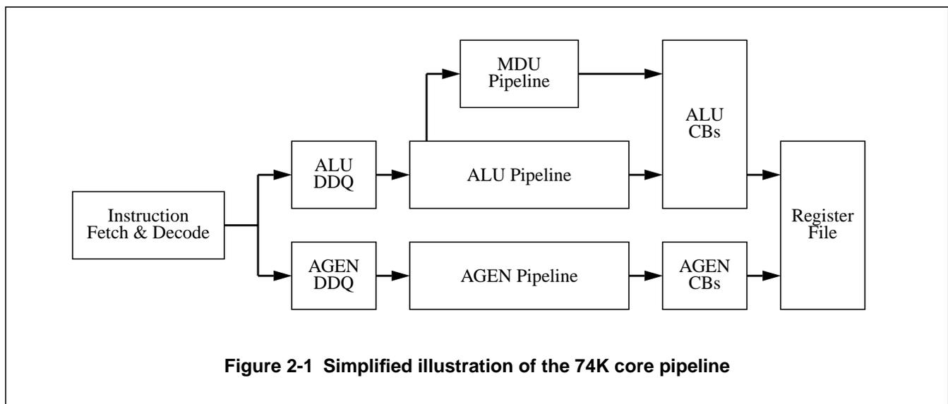
**Figure 2-1 Simplified illustration of the 74K core pipeline**
